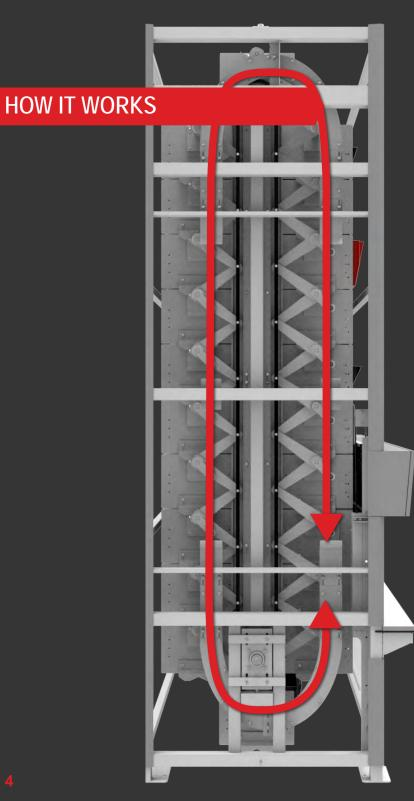
The **Pan Carousel** is designed around the product to person principle, which ensures that the operators no longer concern themselves with search and retrieval functions, but allow the vertical carousel to retrieve items regardless of their location. Carriers are connected to the chain at two separate points allowing the carriers to rotate at the apex and remain 'nested' while vertical to provide maximum space utilization within the carousel.
